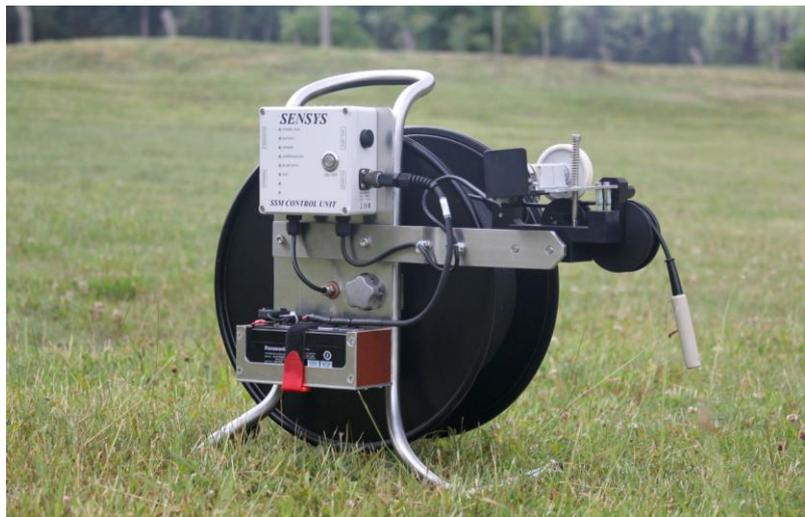
Sensor, length counter, data acquisition and power supply on cable reel
